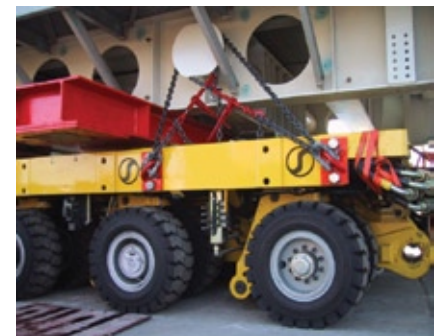
Our site supervision executes quality checks of lashing and stability for comparison with project work pack requirements prior to transportation of the load.
