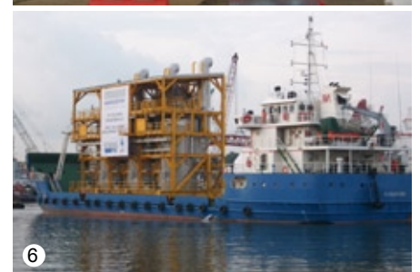
1 to 6 above – Fabrication, overland transport, lifting and marine transport of an LP Boiler module by AOS at their waterfront facility in Singapore.
