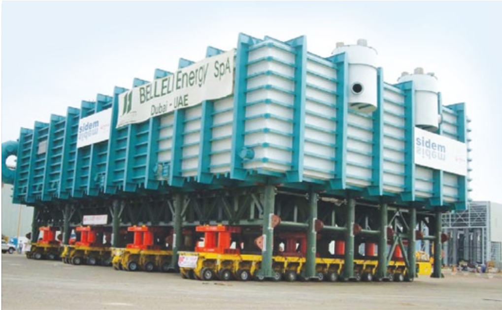
Load out of a 1,700 te MED unit using 64 hydraulic axle lines of self propelled modular trailers (SPMT's).
